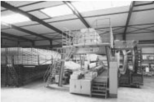
3.4 The highly productive and versatile double rapier Carpet and Rug Pioneer CRP92 weaving machine, made by Van de Wiele. Available in widths of 3 m, 4 m and 5 m.
