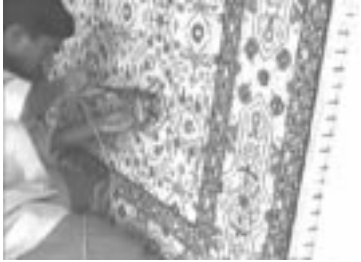
7.43 Hand tufting operation.
